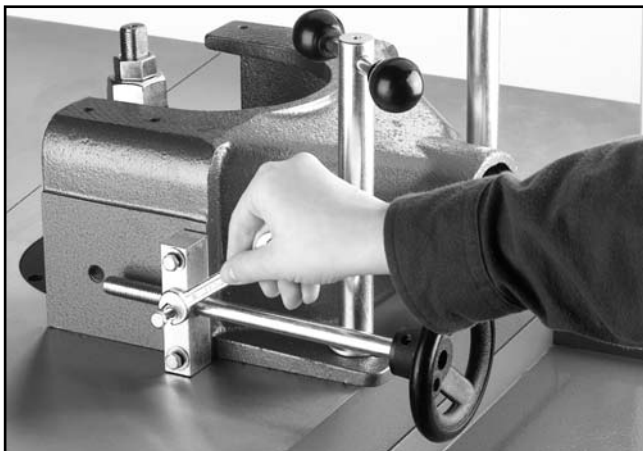
Figure 14. Tightening bolt into shaft groove.
